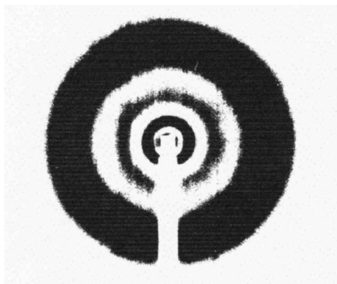
Figure 5. Pinhole camera powder X-ray diagram of the \text{SmC}_1 mesophase of polymer BCDA6BP, showing the two small angle sharp reflections and the wide angle diffuse band.
